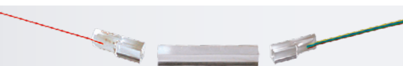
Planar optical waveguide chip with fiber arrays
