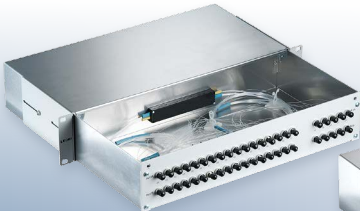
multiple multimode splitter with PCF fibers and ST connectors in a 19" rack
