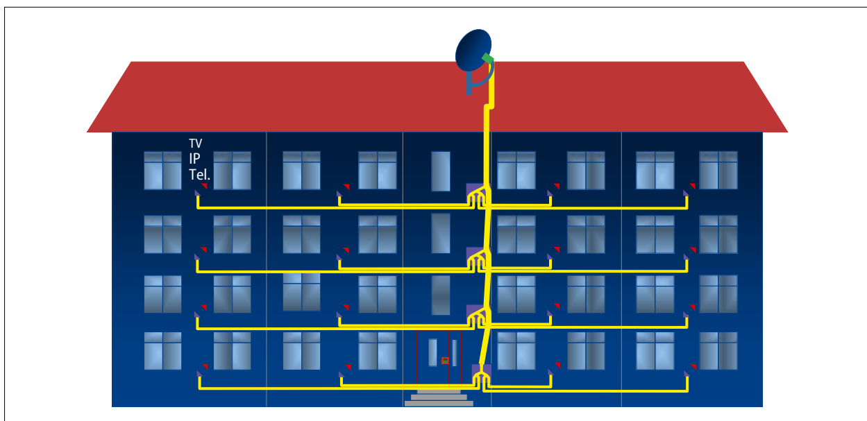
Figure 47: Fiber optic building distribution
