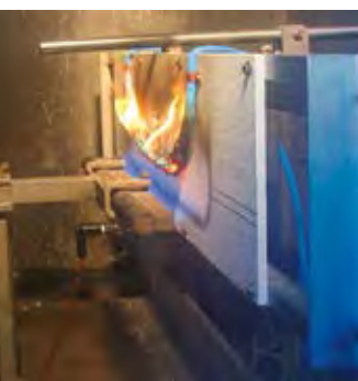
Figure 23: Testing of burning behaviour of fiber optic cables
