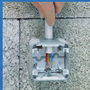
3/ The membrane of the end cap compensates for any misalignment of the tube and ensures IP 55 protection of the installation
