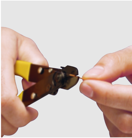
Remove the sheath from the fibre
