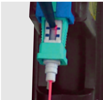
Slide the microswitch on the connector to make the connection
